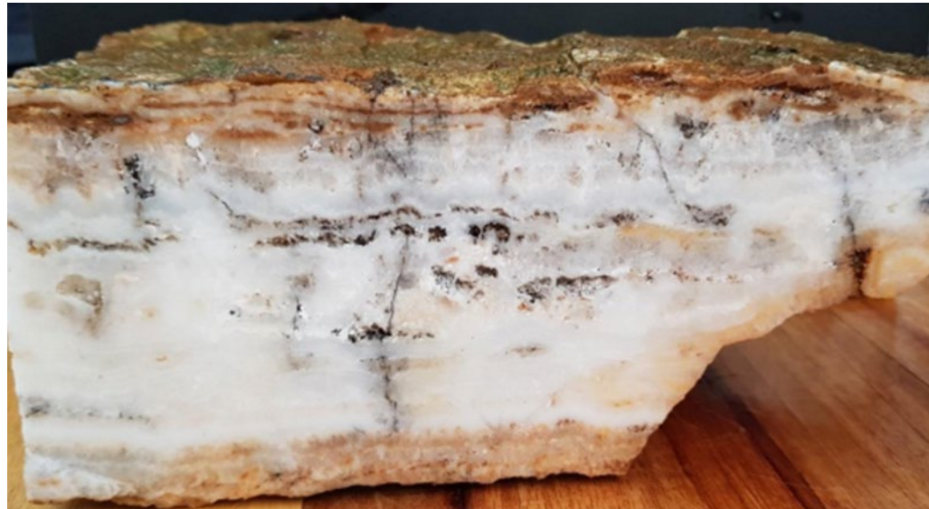
Crustiform and colloform chalcedonic and amethystine quartz – Silver Vein, Talang Santo South
