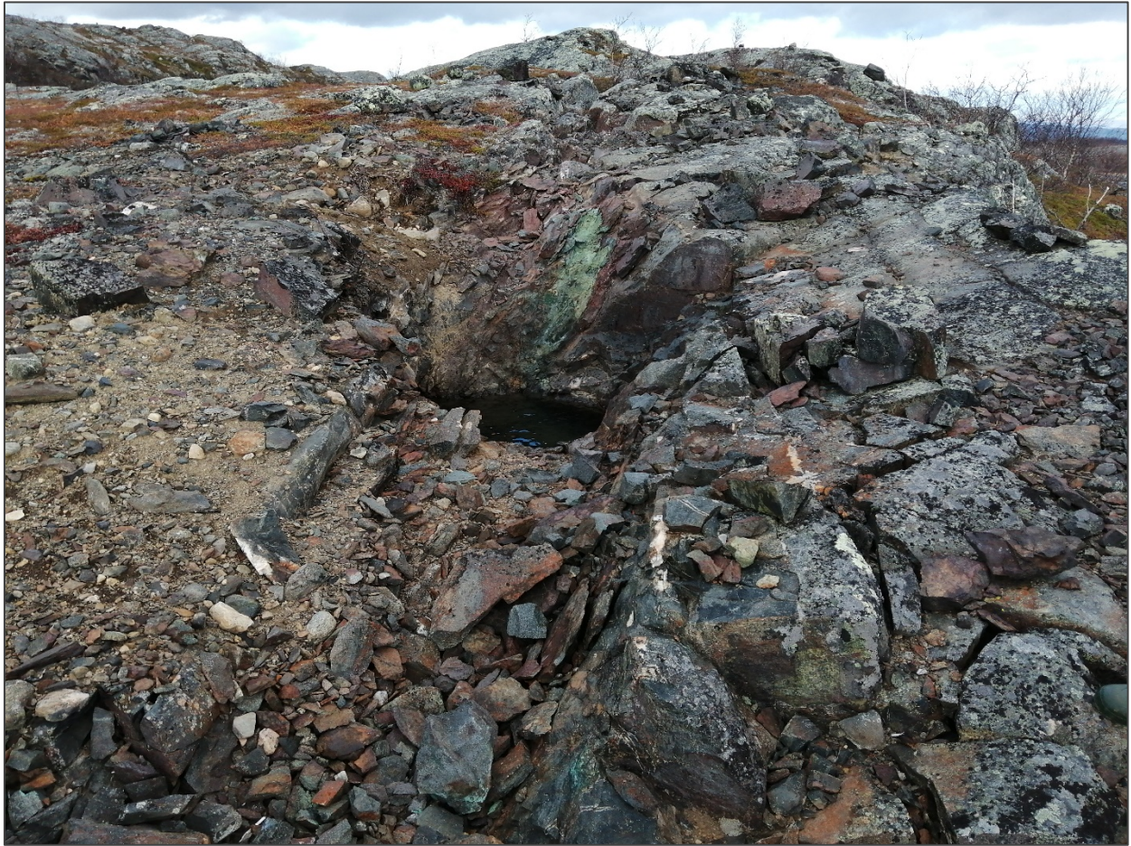
PLATE 2: Shallow shaft at the centre of an artisanal working along the strike of a quartz-copper sulphide vein zone.
